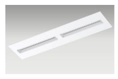
The Micro-louvre G2 is an updated luminaire for those situations where a more discrete ceiling presence is desired. By providing a specific lens and reflector/ louvre cell for each LED package, the light distribution is tightly controlled while maintaining good levels of efficiency. It retains a shallow profile in the ceiling, and there are options for surface-mounting and plasterrecess (with optional frames) in both 600x600 and 300x1200 sizes.
